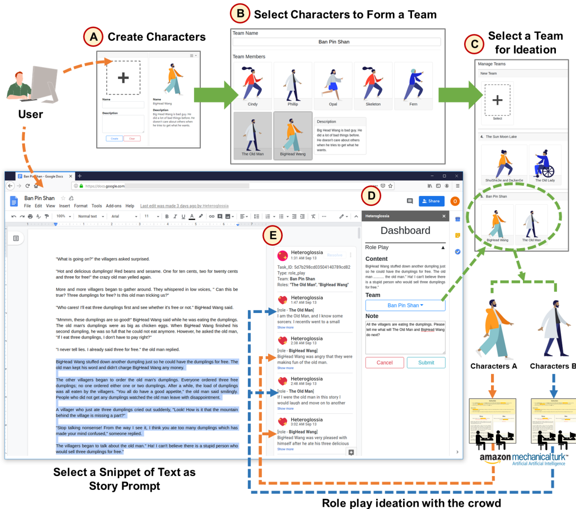
Figure 2. The system overview of Heteroglossia. Heteroglossia incorporates a web site to manage information and a Google Docs add-on for writing. Users start by creating characters (A) and forming teams of characters (B and C) on the Heteroglossia website. After setting up the characters and teams, users start writing their own story in Google Docs. When they get stuck, users can select a story snippet to initiate an ideation task through Heteroglossia (D) and acquire follow-up story ideas (E).
