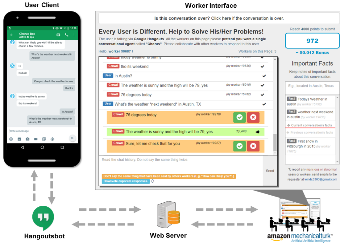
Figure 2: The Chorus interfaces for end users and crowd workers. End users see an interface similar to an instant messenger window, whereas crowd workers see an interface that allows them to see candidate responses, to vote for responses of other workers, and a working memory space. Incentive mechanisms moderate the frequency at which workers are motivated to take different actions (contributing a message, voting for another worker’s message, etc).
